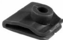
A21615 Maroon nylon M6 (#14) screw size panel range : up to 2mm center of the hole to edge : 12mm bte/box : 15
