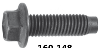
160-148 (N605920-S 2) Phosphate M10-1.50 x 33mm Hex Washer Head With Dog Point Class 9.8; 13mm Hex 20mm (13/16") Washer Head O.D. Ford
