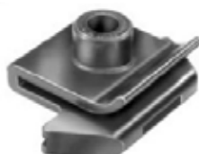
253-1294 Black nylon 5.6Mm (#12) screw size panel range : up to 2mm center of the hole to edge : 9mm bte/box : 10
