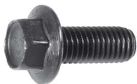
160-150 (N605800-S 2) Phosphate M10-1.50 x 25mm Hex Washer Head Class 9.8; 13mm Hex 20mm (13/16") Washer Head O.D. Ford
