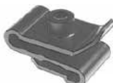
A20956 Black nylon 5.5Mm (#12) screw size panel range : up to 1mm center of the hole to edge : 14mm bte/box : 10
