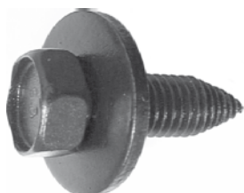
160-175 Phosphate M10-1.50 x 30mm Hex Head Sems * Class 9.8 29mm (1-1/8") Washer O.D. 15mm Hex
