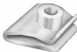
A21614 White nylon M6 (#14) screw size panel range : up to 2mm center of the hole to edge : 12mm bte/box : 15
