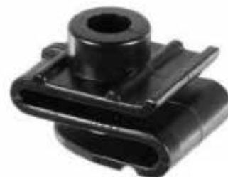
A21378 Black nylon M6 (#14) screw size panel range : up to 1.5Mm center of the hole to edge : 8mm bte/box : 25
