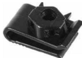
A21459 Black nylon with captive metal hex nut M6 – 1.0 Thread panel range : up to 4mm center of the hole to edge : 14mm bte/box : 10
