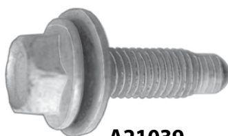
A21039 (11516845) Zinc Organic M10-1.5 x 35mm Hex Washer Head Sems * 15mm Hex 25mm (1") Washer O.D. 22mm (7/8") Washer Head O.D. GM Front & Rear Bumpers, Dash, Doors & General Purpose 1997 - On
